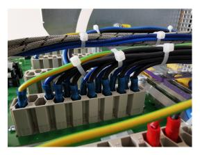
Connect the heating connection cables to Faston blade terminals O1-O6, O1N- O6N and/or O7-O12, O7N-O12N for each backplane.
