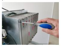
Loosen, remove and store the four locking screws for the moving part of the pT+RACK.
