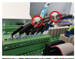
The cable lengths and strain reliefs must be designed in such a way that connections on the low-voltage side (e.g. sensors, etc.) cannot touch connections/contacts on the power section after disconnection and vice versa.
